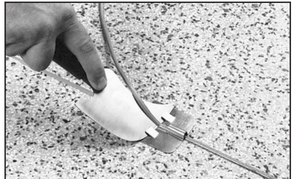
Fig. 51. Trim the welding rod using a spatula guide.
