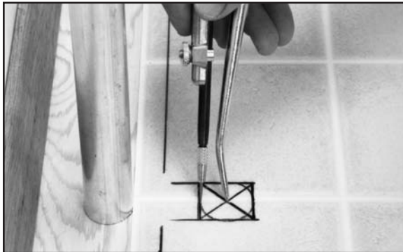
Fig. 70. Scribe a circle with one leg on the center of the X mark.
